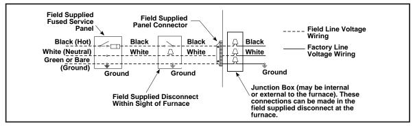
Figure 26. Line Voltage Field Wiring
